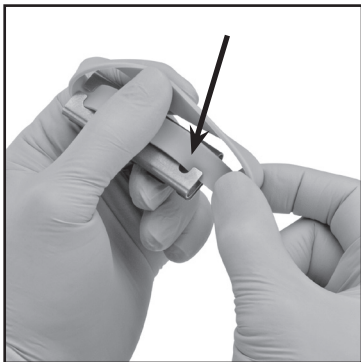
Figure 1. Thread a silicone grip band into T-slots on both ends of organizer.
